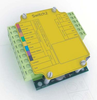
Switch2 is a standalone, single door access control unit from Paxton. A Switch2 control unit is fitted on the secure side of the door, with the reader fitted on the other side. The Switch2 control unit stores all of the access permissions for users' within the unit; meaning that even if the reader is tampered with, the door remains secure.
